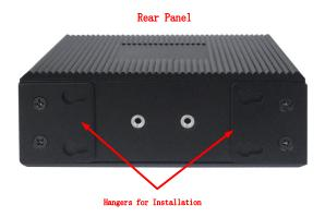
Step1. Remove four mounting fin screws on the back panel as shown below.
